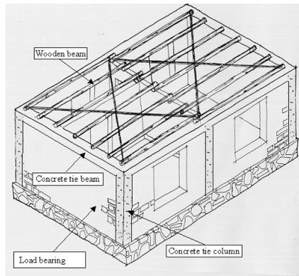
Figure 2A: Key Load-Bearing Elements
