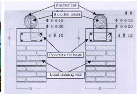
Figure 4B: Wall cross-section showing a concrete tie beam ad roof-to-wall connection
