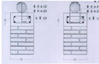
Figure 6A: Illustration of Seismic Strengthening Techniques
