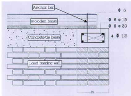
Figure 4C: Wall side view showing a concrete tie beam and roof-to-wall connection
