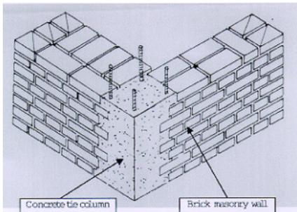
Figure 3: Critical Structural Details: Concrete tie column
