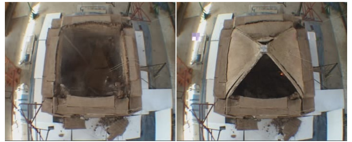
Figure 5. Partial and complete collapse of arched roofs: (b) shake-table tests by Bakhshi et al. (2009)
