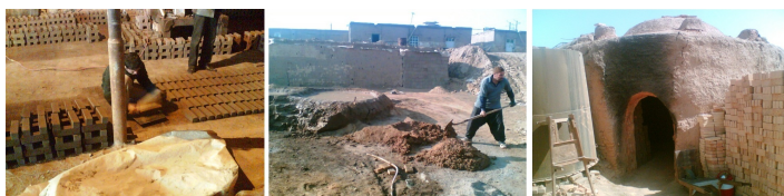
Figure 9. Construction of sun-dried, baked square and rectangular adobe blocks: (c) Tehran province
