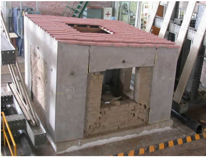
Model tested in PUCP shaking table, with some damage under severe earthquake.
