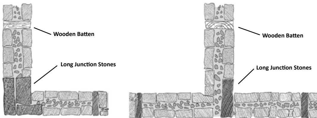
Figure 3.30 Placement of long stones at wall intersections (adapted from: Bothara et al. 2002)
