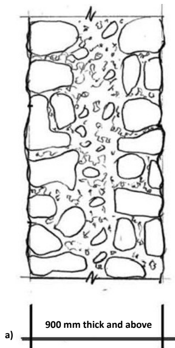
Figure 1.28 Stone masonry walls in Maharashtra, India: a) an uncoursed random rubble stone masonry wall (source: CBRI 1994); b) a semi-dressed stone wall with an exterior wythe built using wedge-shaped dressed stone (Source: CBRI, 1994), and c) an example of a semi-dressed stone wall (photo: S. Brzev)
