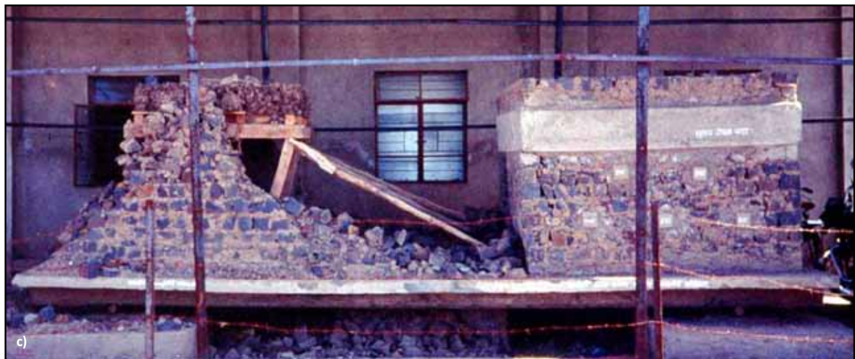
Figure 4.1 Verification of seismic retrofitting methodology for stone masonry buildings through shake-table testing: a) strengthened (retrofitted) model, b) unstrengthened model after testing, and c) models at the end of the experiment (unstrengthened model shown on the left) (source: GOM 1998)
